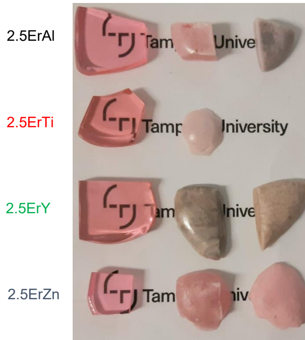
Figure 36. Picture of the 2.5Er glasses before and after heat treatment.
