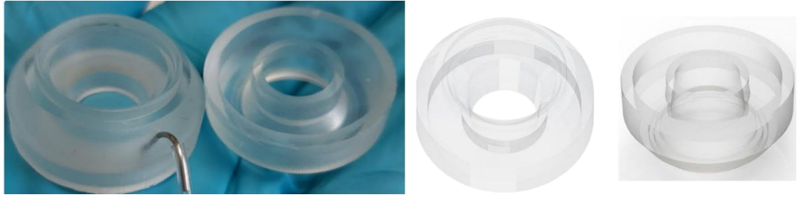
Figure 15. Photograph of a finished device from above and below with the pressure inlet inserted shown on the left, and corresponding CAD-designs on the right.
