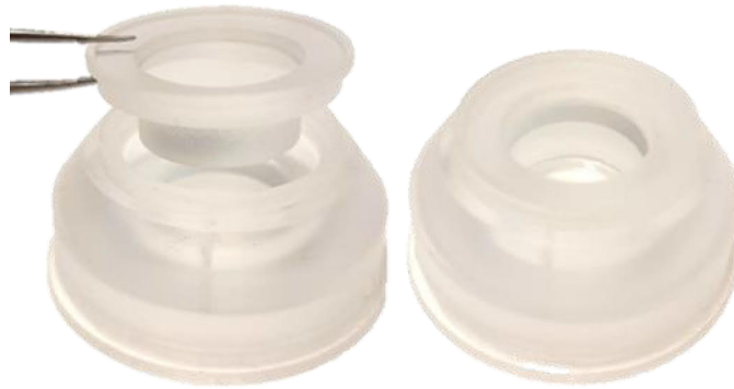
Figure 21. A glass lid is placed on top of the device to prevent the evaporation of media.
