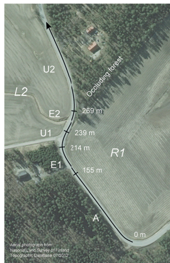
Figure 4. Study II: Aerial photograph with curve phases and their boundary locations from the beginning of the segment. Segment symbols are the following: A = approach, E = Entry, U = unwinding. Phases E1 and U1 belong to curve R1 and phases E2 and U2 to L2. When approaching the right curve R1 along phase A, the forest occludes visibility along the road creating an occlusion point.
