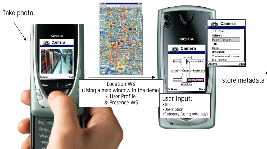
Figure 10. Annotating the photographs. The user takes a photo. The system retrieves the current location from the location web service. The user selects the corresponding category from the ontology browser, and enters a free text description. The system automatically gathers the location and author information. The user accepts the metadata, and it is stored together with the image to the repository.
