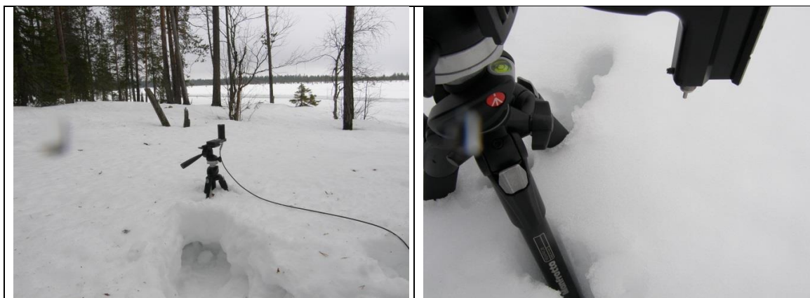
Figure 24. Spectrometer measurements of irradiance (left) and reflectance (right).
