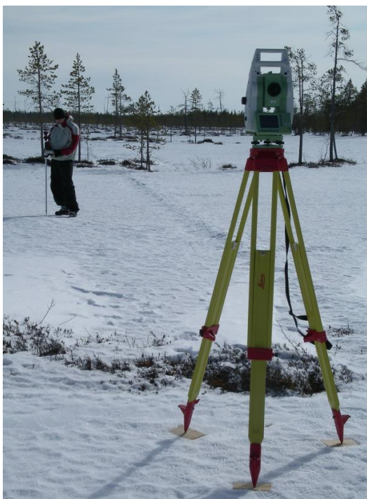
Figure 42. Tachymeter measurements of snow surface roughness.
