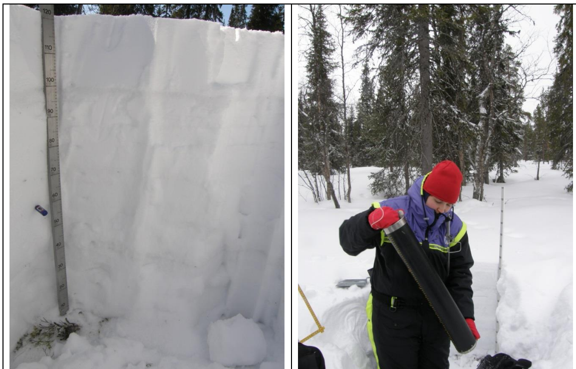
Figure 28. Snow depth, temperature profile and snow water equivalent measurement.
