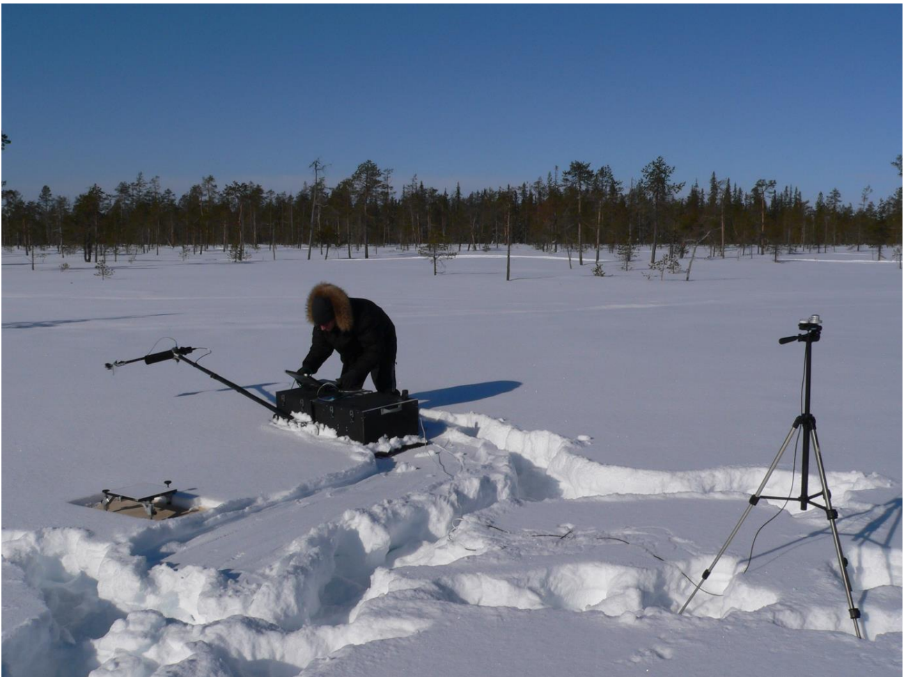
Figure 53. FIGIFIGO measurements in Mantovaaranaapa 22.4. 2010. The measurement spot is 50 cm in front of the black box. Foreground left the Spectralon standard, right pyranometer monitoring skylight. The snow is a couple of days old, quite loose and smooth surface.
