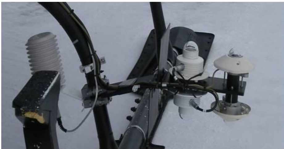
Figure 12. The pyranometers and the UV sensors attached on one side of the helicopter. A similar pair is attached to the opposite side. The Pt100 thermometer and the Humicap-sensor are on the left.
