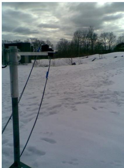
Figure 1. Year 2009: The first version of the portable setup for snow albedo measurements with the Bentham spectrometer.
