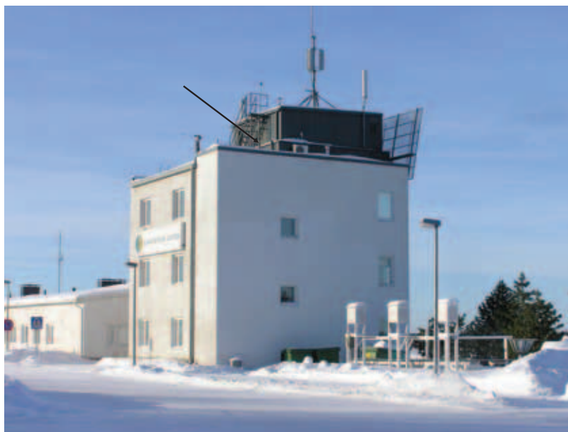
Figure 1. Aerosol sampling station at the Rovaniemi airport, regional office of the FMI. The arrow points to the sampling inlet on the roof of the building.
