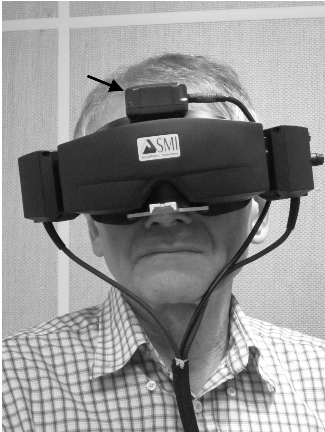
Figure 4 A subject wearing the VOG mask showing the integrated head-position sensor on top of the mask (arrow).
