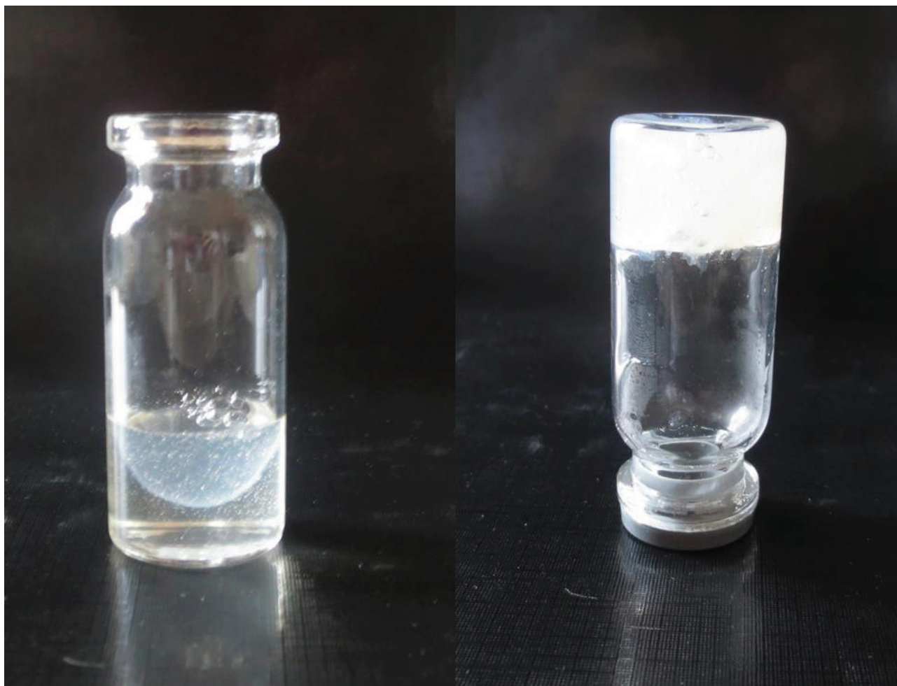
Figure S5. Photographs of chitosan solution added to alginate solution (left) and gel instantaneously formed after stirring (right).
