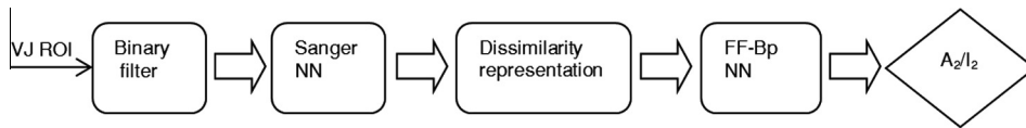
Fig. 2. In the block diagram the input (VJ ROI) is the region of interest extracted by the Viola-Jones algorithm; the ROI is first binarized and then coded through an Sanger neural network into a vector of 16 components. A dissimilarity representation based on the Sanger components is finally computed and passed to a trainable classifier which decides about the attentive ( A_2 ) or inattentive ( I_2 ) state of the driver.
