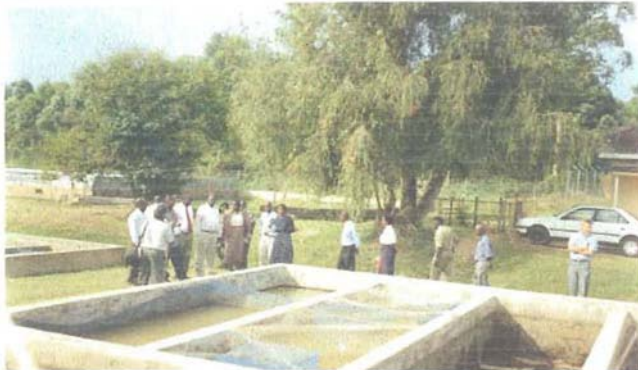
Concrete ponds as alternatives to earthen ponds. Experimental work at Kallansi ARDC
