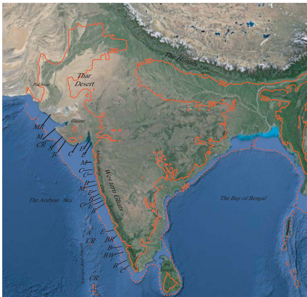
Figure 8: Map depicting the most significant coastal features along the West coast of India (modified from Mukhopadhyay and Karisiddaiah, 2014). The continuous red line indicates 200 m height contour and the dashed red line shows the 200 m depth isobaths. The main features are: A-Archipelago; B-Beach; BR-Beach/Dune ridges; BW-Backwater; C-Cliff; CR-Coral reef; E-Estuary; M- Mangrove; MR- Marshland.
