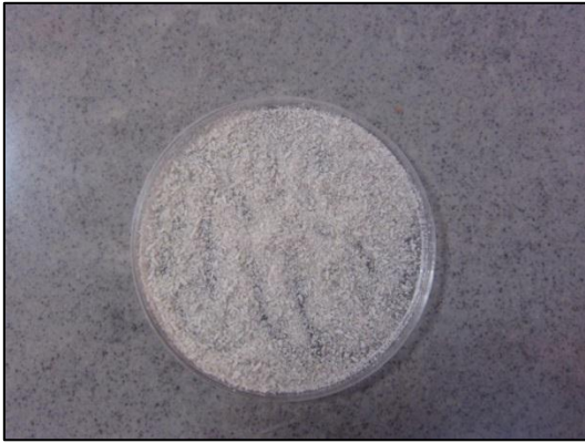
Fig.4.8. The trimmed spines were fragmented in liquid nitrogen with pestle and mortar
