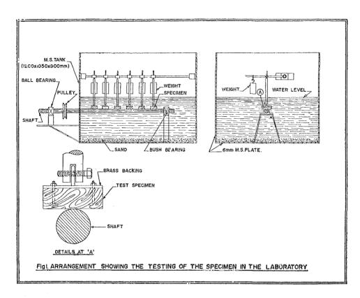
tank of size  $120 \times 105 \times 90$  cm in which the specimens were subjected to wearing by loading them with weights suspended on a lever as shown in the Figure 1.
