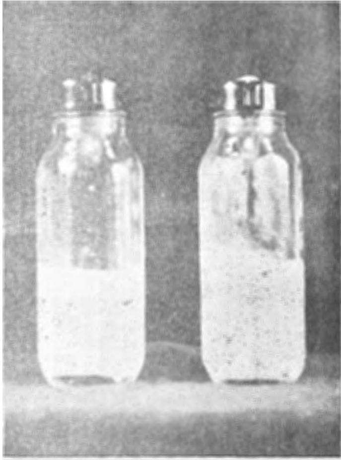
PLATE 2. (a) The angle of jelly in the bottle attached in vertical position to the otter boards. (b) The angle of jelly in the bottle attached in horizontal position to the otter boards.
