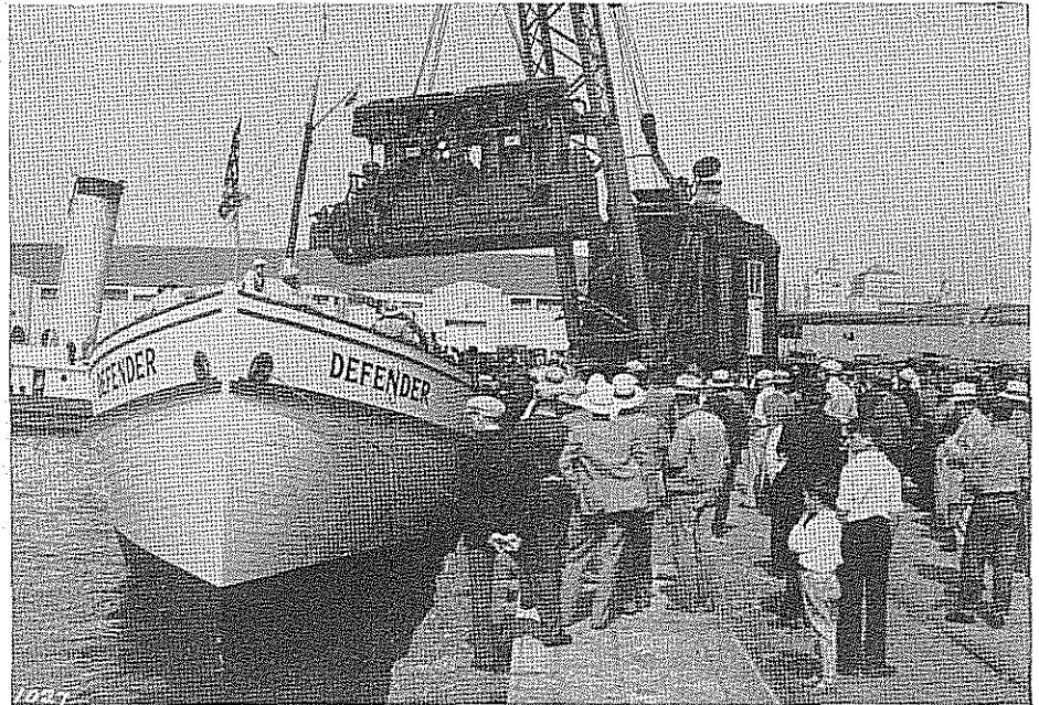
Lowering the 6-cylinder, 350-h.p. Union diesel engine into the Monise brothers new tropical cruiser. The "Defender" has all Union machinery, including the auxiliary plant. One cannot but speculate on what hundreds of thousands of miles this vessel will travel before its years of useful service are done. No Union diesel ever installed in a fishing craft has yet worn out.
