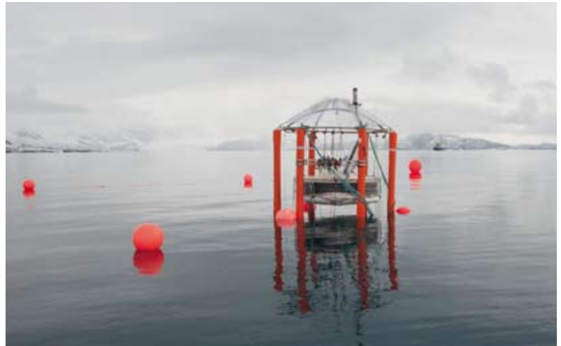
2.5 > In order to determine the effect of increasing atmospheric CO 2 concentrations on the ocean, an international research team enriched seawater with CO 2 in floating tanks off Spitsbergen, and studied the effects on organisms.
