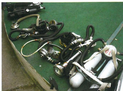
A MEDI Hydromat, homemade double-hose regulators, MEDI full-face mask, and a MEDI 713 (their first sports diver rig, called "Horse lung" due to the breathing work it required).
