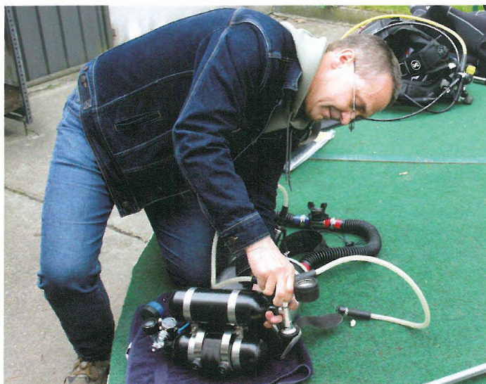
(Below left & right) Self-made rebreather with Poseidon regulator as bailout, made by Lutz Droessler, who is shown preparing his rebreather for a dive.
