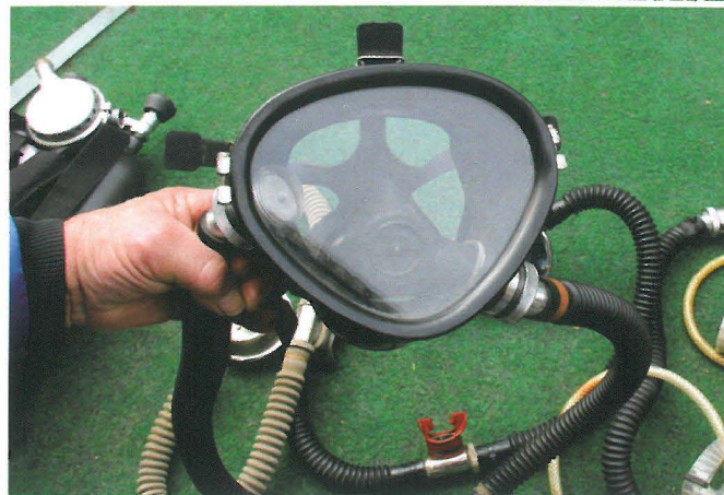
(Left) Czech full-face mask with window wiper. The same mask is shown in the HDS Czech Republic logo.
