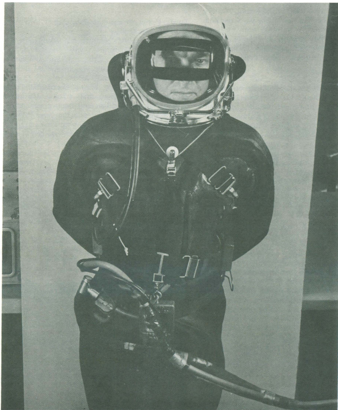
MCI engages in research and design in the area of heated diving suits. Shown above is one of MCI's heated wet suit designs. Hoses at bottom are supply and return for heated fluid which circulates through capillaries built into wet suit. Heated fluid is surface-supplied.
