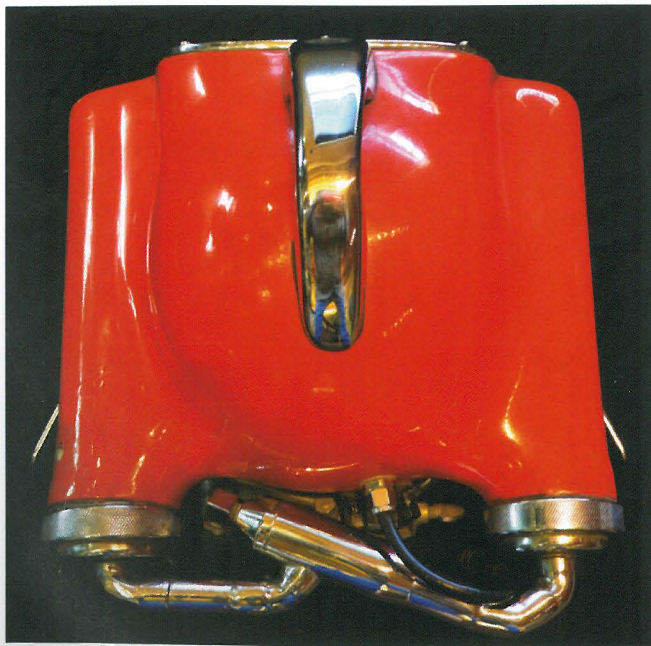
(Above) The plan view shows the venturi jet system plumbed between the scrubber canister's fill caps. 1995.
