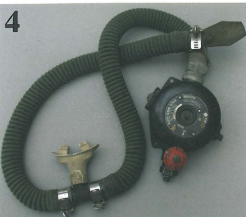
PHOTO 4: The regulator in photo 4 has a flapper valve on the end of a long exhaust hose designed to keep the exhaust bubbles away from the diver's view. The unit could be fitted with an attachment for mounting on a single tank, or onto a manifold for dual surplus oxygen tanks to be used as air tanks for diving (Leslie Leaney Collection).
