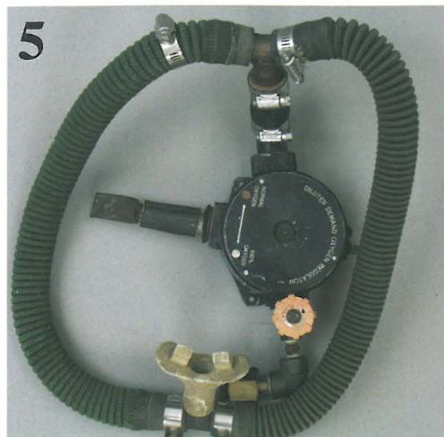
PHOTO 5: This regulator features inhalation and exhalation (from and to) the same demand air chamber in the regulator. A relief valve was placed on one side of the demand air chamber for exhaust, but frequent water contamination of the demand air chamber made it high maintenance and risky for failure. This particular regulator was made to the specifications and instructions found in Popular Science , July 1953. It was designed to attach to a surplus single oxygen tank used as an air supply tank for diving (Leslie Leaney Collection).
