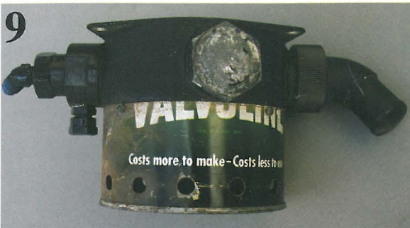
PHOTO 9: Homemade rules! A Valvoline oil can used in an attempt to fit a cover for the Diluter.
