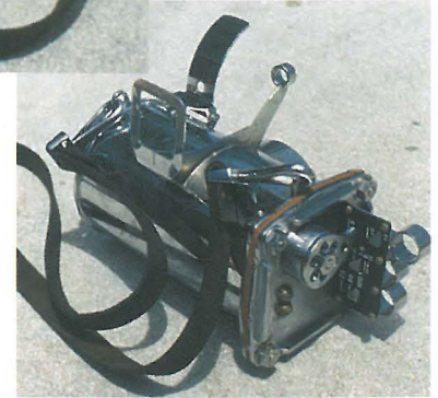
(Above and right) Ivor's viewfinder. The square frame is held up to the diver's face mask. Note the push-pull controls and scales on the right side plate of the housing.
