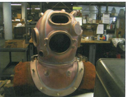
8) Nearly completed helmet and breastplate.
