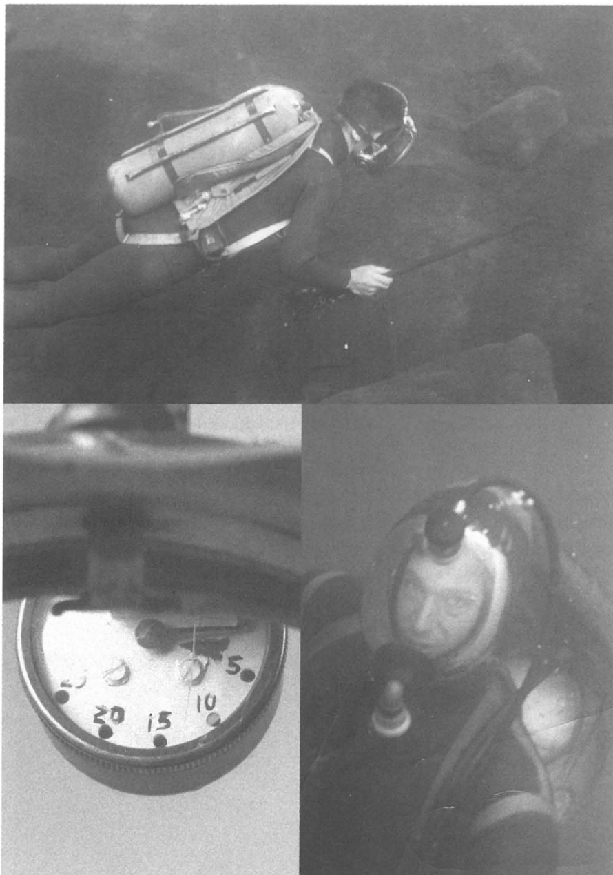
Top: Dad diving with Mae West used as a BC and weights welded to tank frame. Left: Prototype mask with pressure gauge. Right: Bubble mask.
