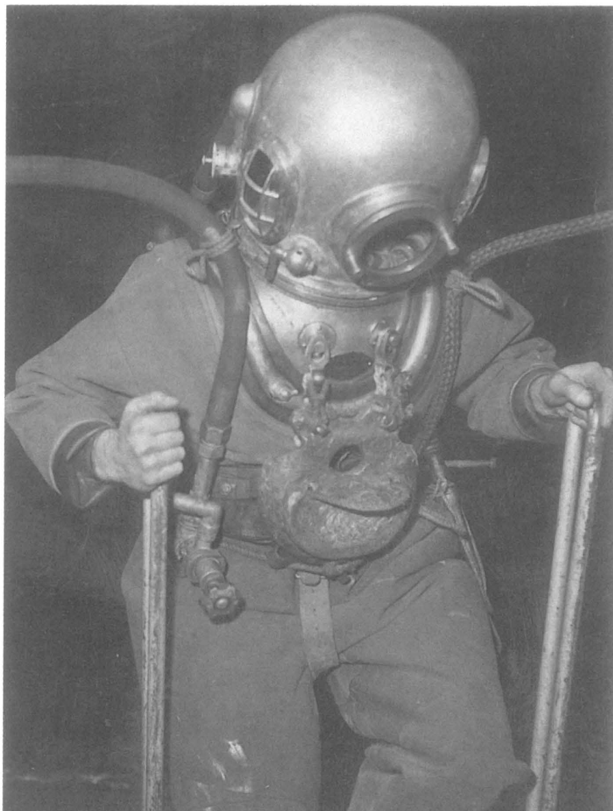
George diving standard navy dress. Note chest weight and hose and line tie-offs.
