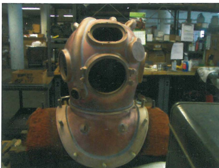
8) Nearly completed helmet and breastplate.
