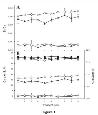
Transects of (A) Sr/Ca atomic ratio and (B) Ca (circles) and Sr (triangles) as atomic percentage when Sr is measured on the PET crystal (solid symbols) and on the TAP crystal (open symbols). Error bars represent 95% confidence intervals.
