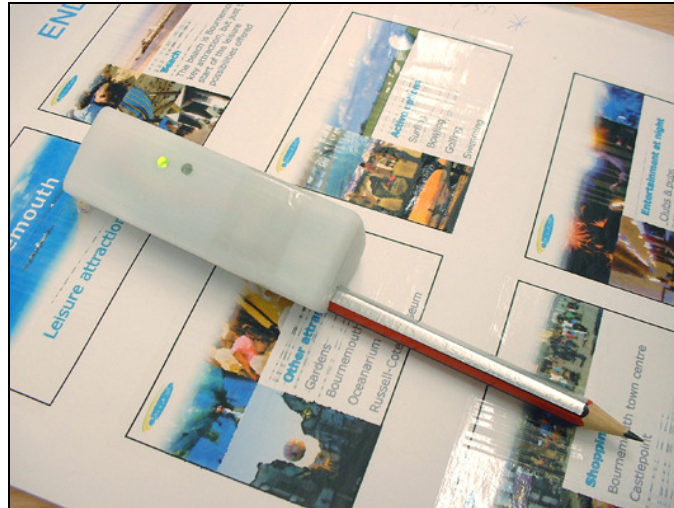
Figure .30 Wireless pencil module shown activated, with external foil contact strip on pencil.
