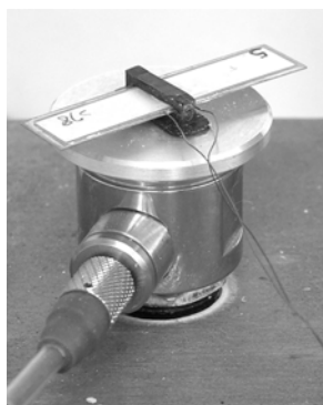
Fig. 3 The SLDMA mounted on an aluminum plate that is screwed rigidly into a force transducer
