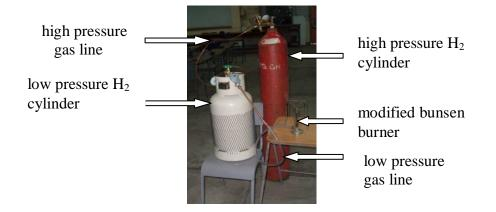
Figure 4.16 Hydrogen Gas Cascading Storage System (CSS) attached to Burner
