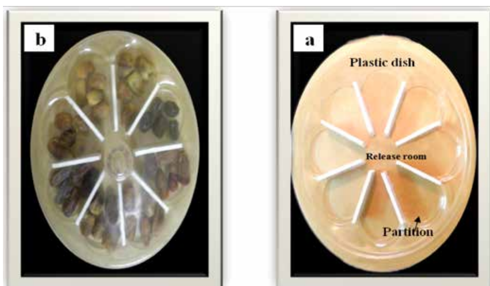
Fig. 1. Arena design which used in preference test (a) = Structure of arena; (b) = Arena during experiment
