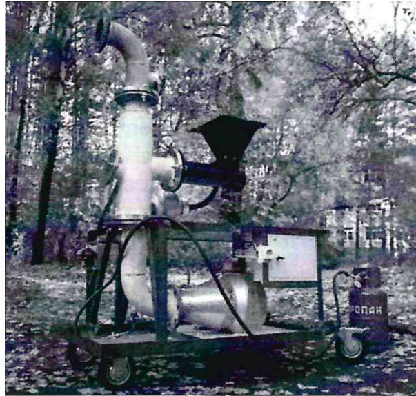
Fig. 1. Setup for producing burning and glowing firebrands.
