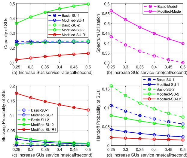
Fig. 2. Performance metrics of SUs for SUs' service rates.
