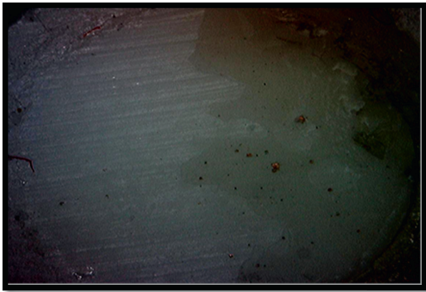
Fig. 5. Stereomicroscopic image of the zirconia fractured sample demonstrating combined adhesive/cohesive failure mode (X = 60).
