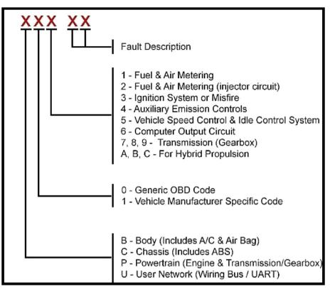
Fig. 2. OBDII Diagnostic codes [17].
