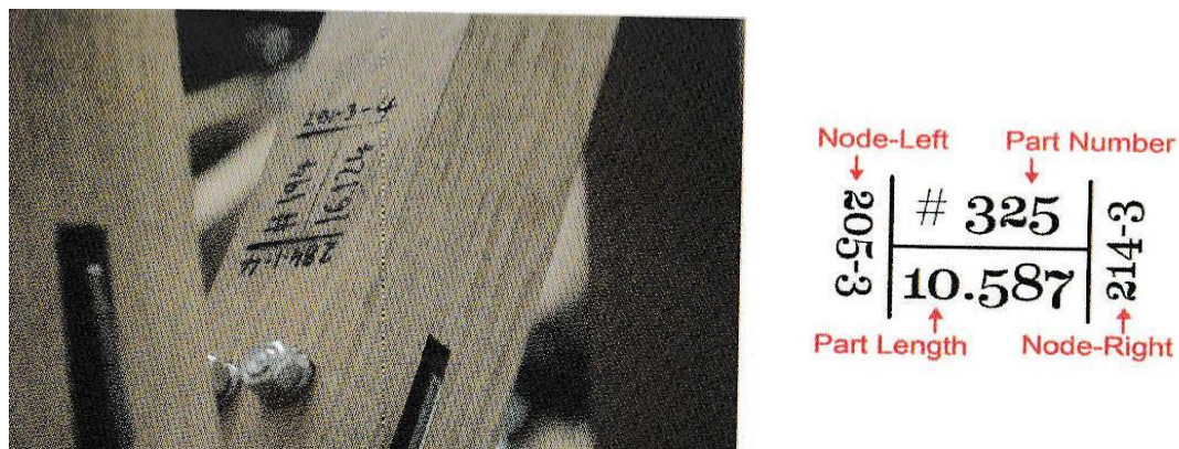
Fig.07 Photograph and diagram showing the Joints labelling system used to guide all manual fabrication and assembly Photographed by Virginia Tech Center for Design Research. Reference: Page 369, Robotic Fabrication in Architecture, 2016
