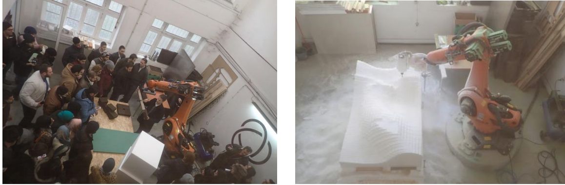
Fig. 5 Gathering with students at the fabrication lab for explanation of the restrictions between design and production processes (left) and stage of fabrication of the milling class project where a block of EPS is being machined by the robot (right).
