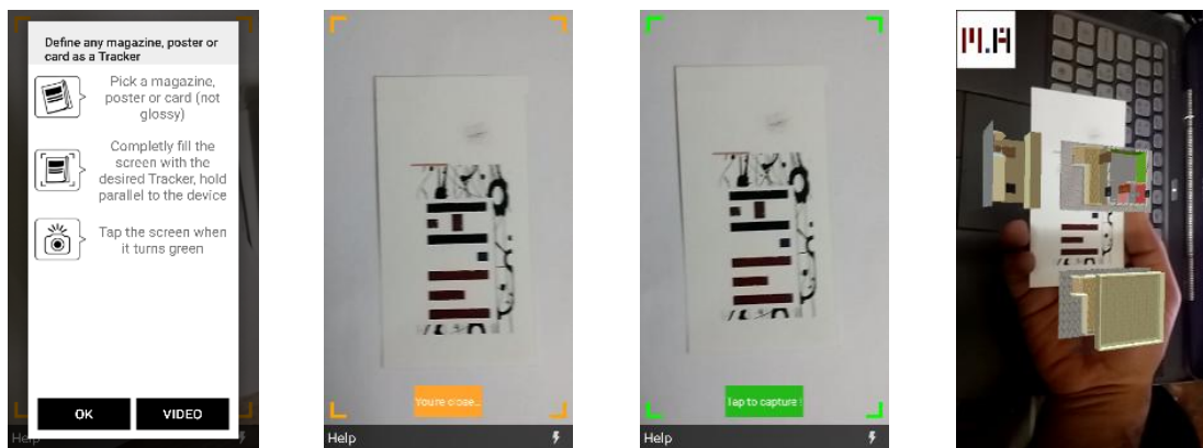
Fig. 3: The process of making new custom tracker for any 3D model Source: Authors
