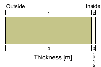
Figure 3 Cross-section scheme of sandstone wall that shows layers and thickness of the assembly Reference: the author
