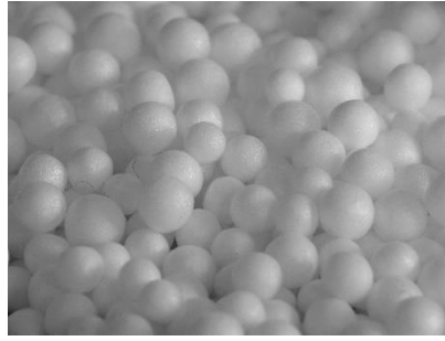
Fig.1: Crushed waste polystyrene particles (5mm diameter)
