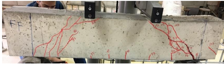
Fig.12: Beam (B4) at failure
