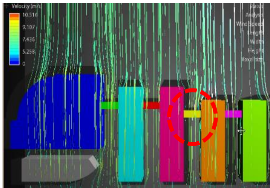
Fig. 4: Wind tunnel simulation between BAU building's blocks (wind speed 5m/s) Source: Authors
