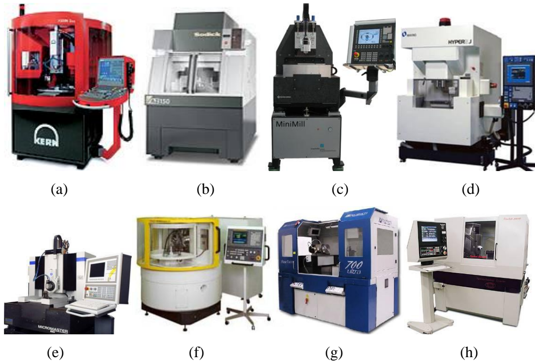
Fig. 2. Industrial precision machine tools with micro milling capability: (a)Kern micro [16]; (b)Sodick AZ150 [17]; (c)Fraunhofer IPT Minimill [18]; (d)Makino Hyper2J [19]; (e)Kuglar MicroMaster MM2 [20]; (f)Fanuc ROBOnano [21]; (g)Precitech freeform 700 Ultra [22]; (h)Moore Nanotech 350FG [23]
