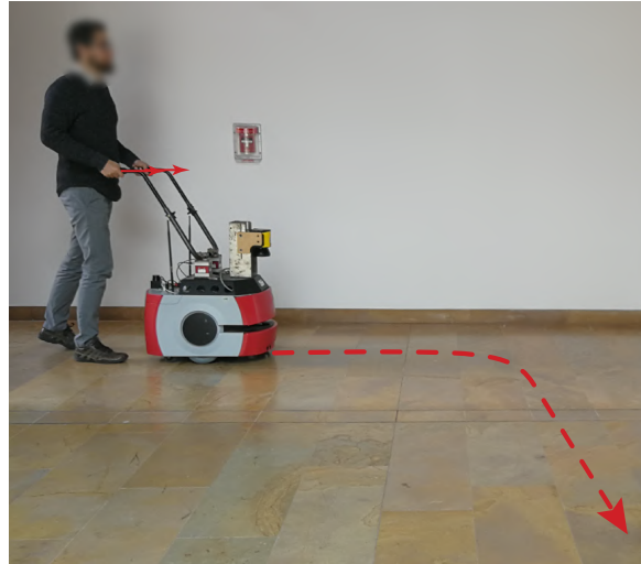
Figure 4.3: Preliminary experiment for the validation of the filtering processes. The user was asked to follow an L-shaped path. Red arrows illustrate impulse forces exerted by the user.
