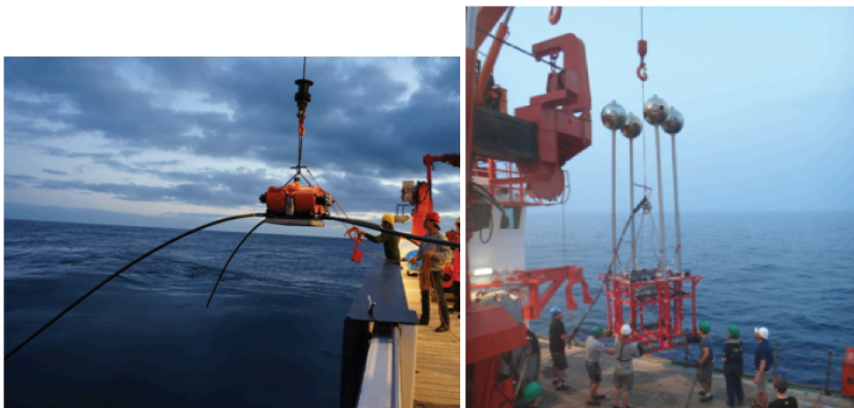
Figure 5.1.1: The Time Domain Electric Dipole-Dipole system consisting of OBEM receivers (left) and the Sputnik transmitter (right).
