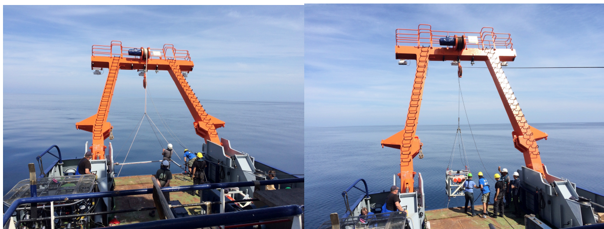
Figure 5.1.6: Deployment of Octopussy. Left panel shows the deployment of the 4x4 m transmitter/receiver coil, right panel the GFK frame on which the instrument's electronic devices were installed.
