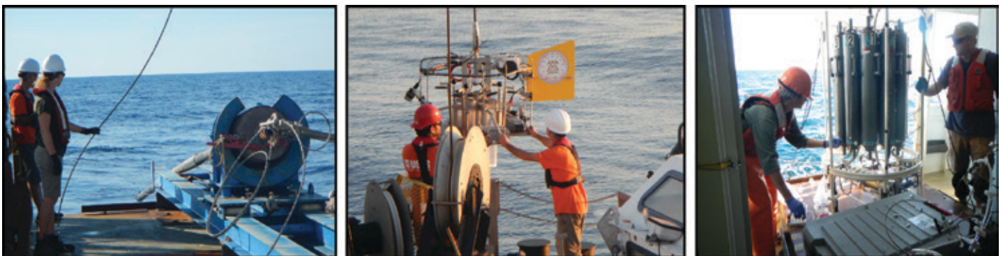
Figure 3. Sampling activities carried out in September 2015 aboard the R/V Sharp . (Left) USGS operational personnel preparing to put the piston corer over the side. (Center) Deploying the mini-multicorer, which was equipped with USGS-built real-time video system. (Right) F. Colwell and S. Krause sampling the CTD.
