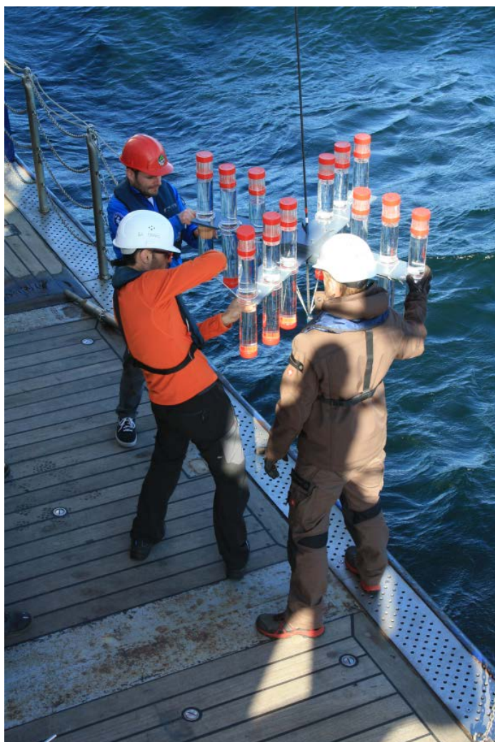
Figure 5: Preparation of the drifting sediment trap with a total of 12 collection tubes per depth during AL 458.
