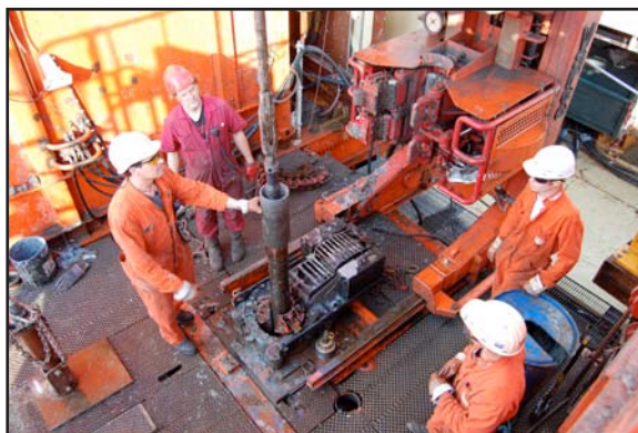
Figure 3: Drill floor on board REM Etive, with the FPC being loaded into the drillstring prior to lowering and coring.
