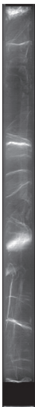
Figure 4: An X-ray of a pressure core collected on Expedition UBGHI showing gas hydrate in veins and layers. Gas hydrate was present at all three locations.
