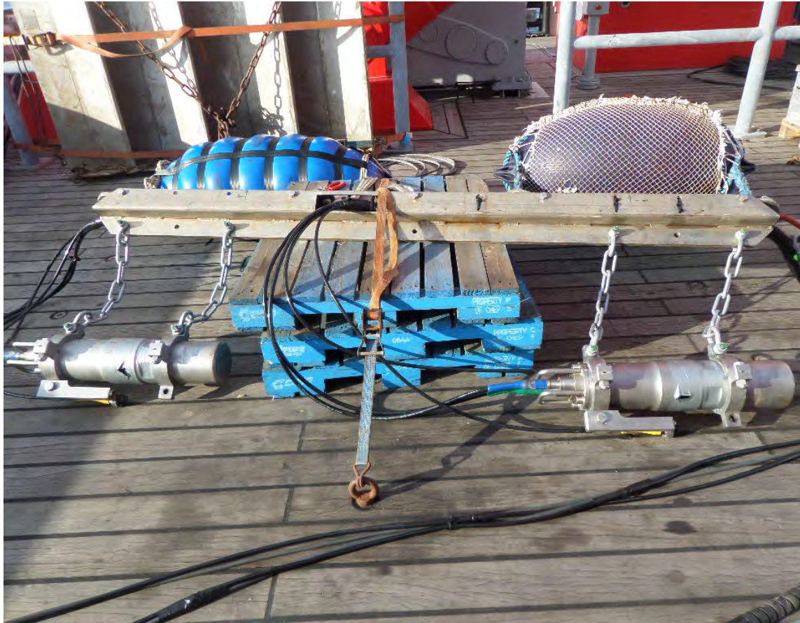
Fig. 6.1.2: Two standard GI-Guns (105/105 in 3 ) in harmonic mode were operated as seismic source during SO241.
