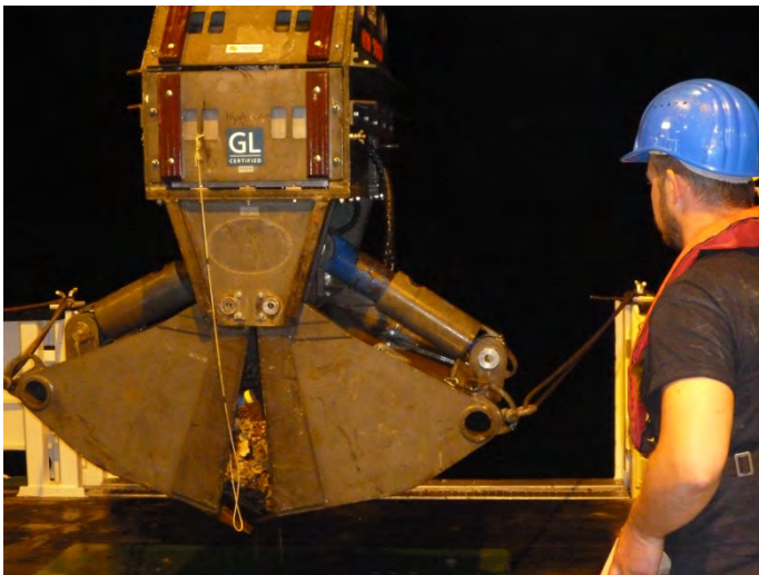
Fig. 6.6.2: The VGHG system after successful deployment on RV SONNE (station 17, VGHG-2). The incomplete closure reflects the blocking carbonate load.
