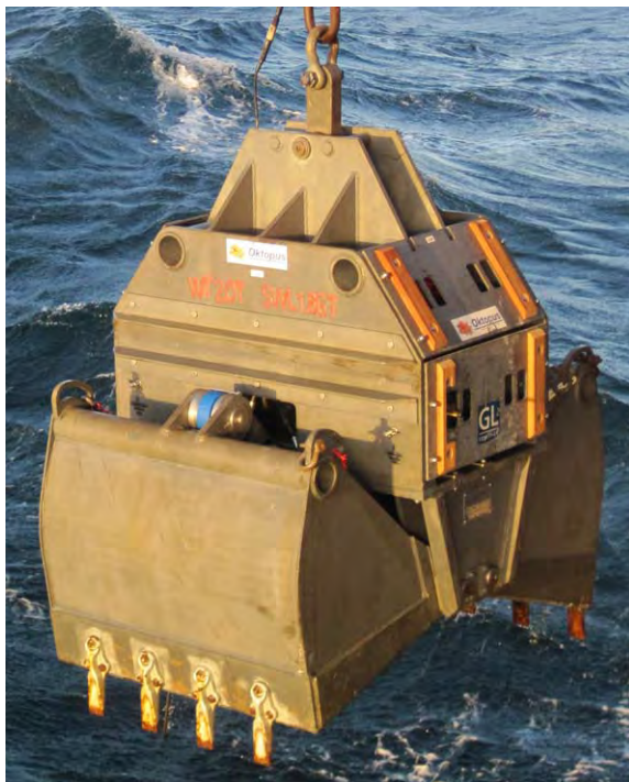
Fig. 6.6.1: The GEOMAR video guided hydraulic grab (VGHG).
