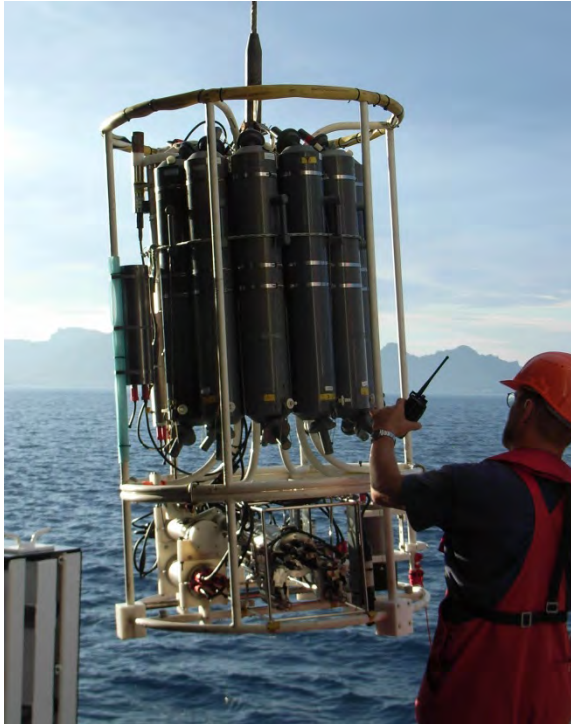
Fig. 6.7.1: Water sampler (11x10 L Niskin bottles) rosette, including Seabird SBE9plus CTD, SBE O2 sensors, Wetlab fluorescence and turbidity sensor, altimeter, Kongsberg-CONTROS HydroC™-CO2 and HydroCplus-CH4 sensors.
