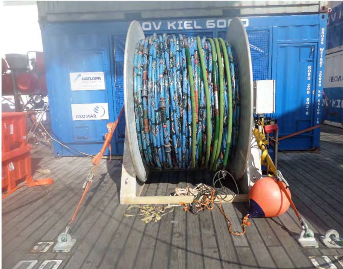
Fig. 6.1.4: GeoEel streamer segments of 12.5 m length were connected to build up the 2D streamer system.
