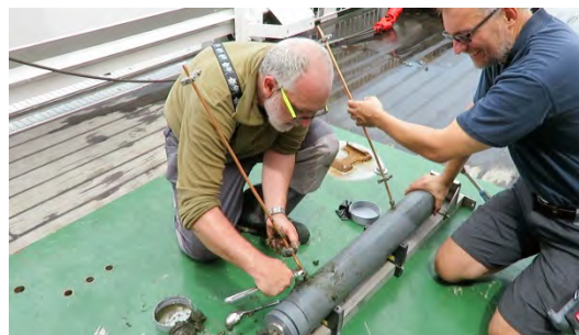
Fig.6.8.1: Left panel. Portable GE-MIMS (black case (< 100l), 40kg, < 40 W) connected to a Niskin-bottle of a CTD probe.
