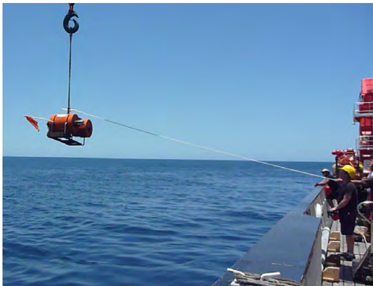
Fig. 6.7.4: ADCP LANDER deployment from starboard side of RV SONNE (free falling deployment).
