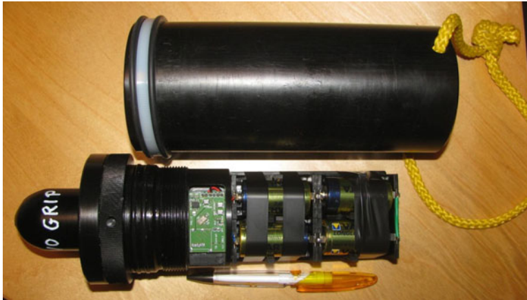
Figure 1. Self-contained synthetic porpoise signal generator “PAL” (dimensions: 30 cm long, 9 cm diameter). Top: the housing is made of 10 mm polyoxymethylene. Bottom: programmable electronics board with protruding omni-directional signal transducer (> 1 month autonomy).
