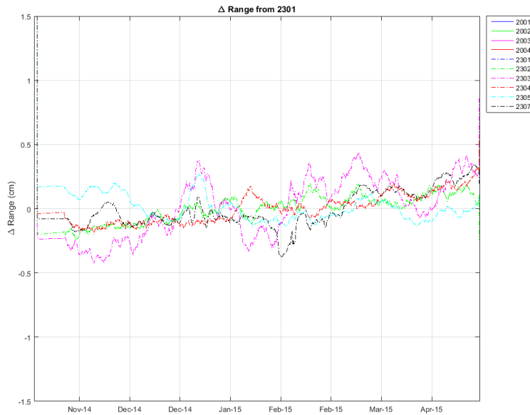
Figure 9: The relative baseline changes from transponder 2301 was calculated using the temperatures from unit 2301 and the Chen and Millero equation to generate the sound speeds. The average pressure for each unit is used, and a salinity of 38.4 psu. The results are filtered, most of the spikes due to temperature episodes are gone but some remain perhaps due to the time response and a genuine salinity change.
