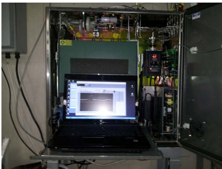
Figure 10.3 Automated flowing pCO 2 measuring system.
