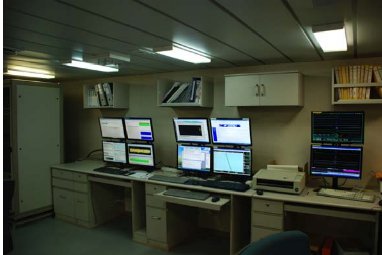
Figure 3.5 The seismic survey control system including navigation, airgun controller, bird controller, recording system and quality control system in Main Dry Lab.
