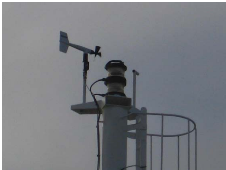
Figure 11.4 Windmill anemometer at the foremast of Araon
