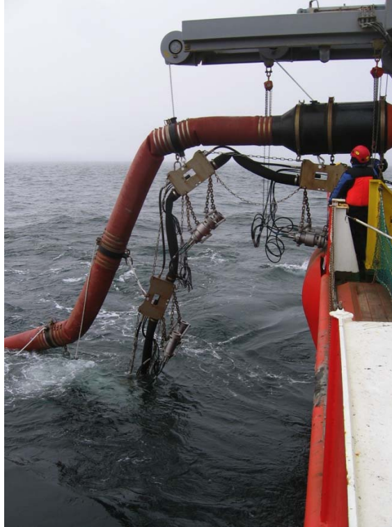
Figure 3.3 The airgun array launching into the Beaufort Sea.
