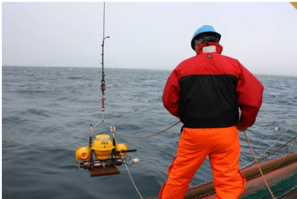
Figure 4.3 Graham Standen operating the release-hook while deploying OBS from the stern of the Araon.
