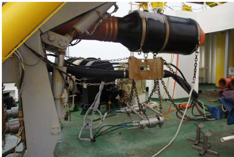
Figure 3.2 Airguns attached on the airgun array.
