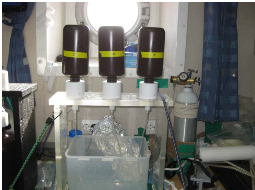
Figure 10.6 Nitrogen gas purging system for collecting DOC and POC.
