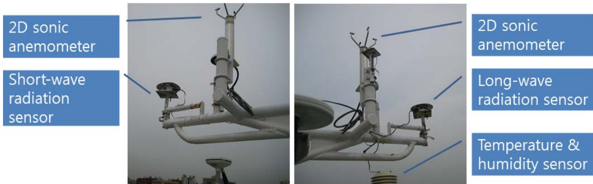
Figure 11.2 Instruments located on the radar mast of the Araon. Note that 2D sonic anemometers provide wind information for the cruise only.
