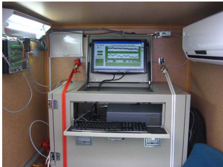
Figure 11.6 Cavity ring-down spectroscopy analyzer in the shelter.
