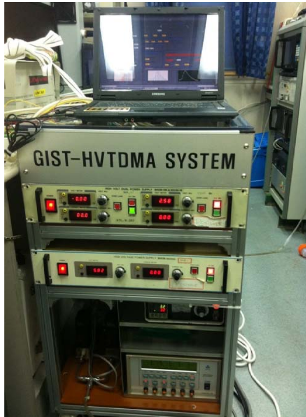
Figure 11.11 HVTDMA system operated on the Araon.
