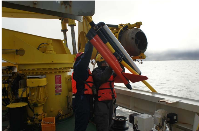
Figure 3.4 The streamer is launched. The cable-leveller (bird) is attached to the streamer and tested.
