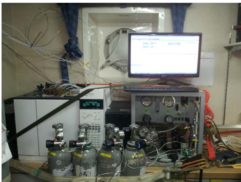
Figure 10.4 Gas chromatography system for measurements of CH 4 and N 2 O.
