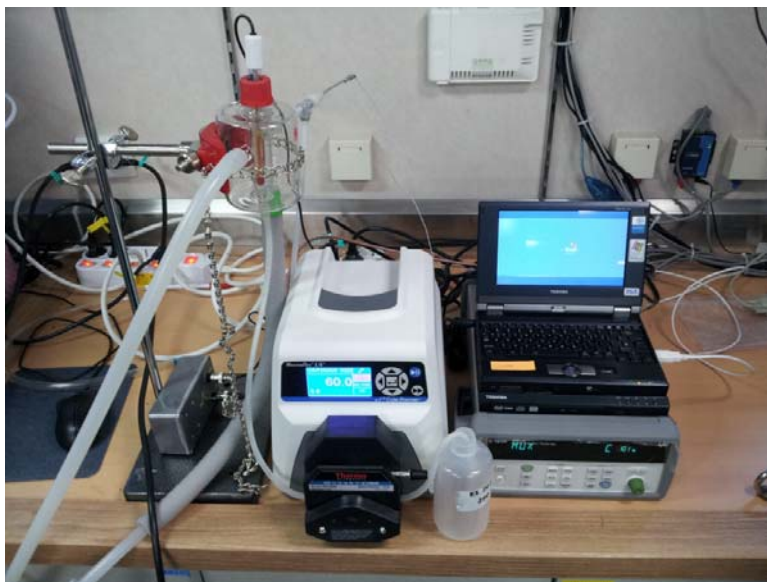
Figure 10.2 pH measurement system.
