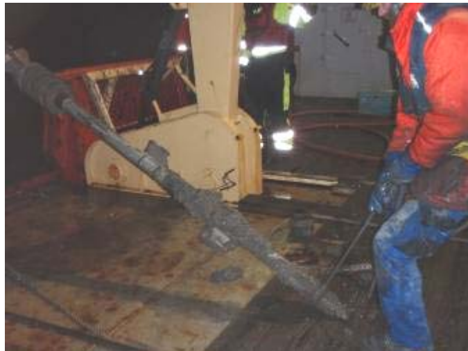
Figure 3. Image of the gravity core recovered on deck, showing outriggers used for the MTL loggers. Note the amount of sediment on the outside of the core-barrel which was used to identify the apparent penetration of the tool.
