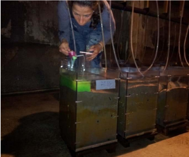
Figure 8: Dr Ana Queiros (PML), benthic ecologist, layering the fluorescent tracer used for the bioturbation assessments carried out during the high CO 2 and formation water mesocosm experiments (NIVA's marine research station, Solbergstrand). The sediment mesocosms can be seen on the floor, with tubing providing input for the experimental water treatments. The experiment lasted 20 and 3 weeks, respectively.
