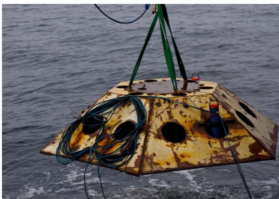
Fig. 5.5.1 Left: MASOX seabed observatory recovered. Clearly visible are the two Seaguard RCMs and the thermistor chain. Right: Schematic drawing of the observatory and its instruments.
