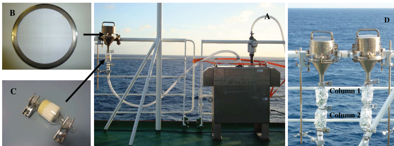
Figure SI 1. High-volume air sampling on board F/S Polarstern . Picture A shows the entire operation system; picture B shows the stainless steel filter plate with a GFF filter; picture C is the glass column (Length: 16 cm, O.D. 6.0 cm, I.D.5.2 cm) packed with 30 g of PAD-2 resins (Particle size: 0.3-1 mm, Surface area: 450 m 2 /g) and a slice of polyurethane form (2.5cm x 5 cm); picture D shows sampling with two columns for breakthrough check. The column is always wrapped with aluminum film during sampling to prevent from sunlight.
