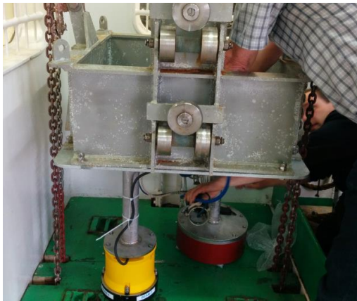
Figure 3: Mobile installation of the EM2040c multibeam transducer (red) and the 300 kHz RDI ADCP (yellow) in the moonpool; 19.10.2014, R/V ALKOR
